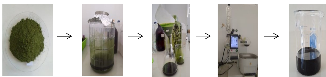
Figure 3. Extraction process of papaya leaves using maceration method
