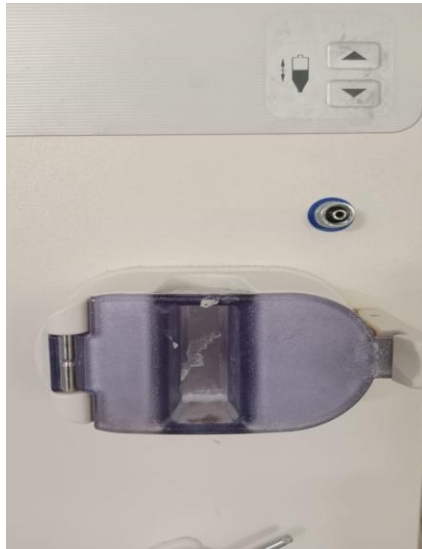
Gambar 10 Venous Clamp Sensor
