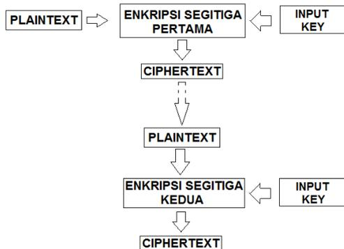
**Gambar 6.** The encryption scheme of the triangle chain cipher
