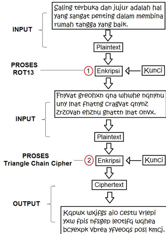
**Gambar 2.** Data input, Process and output Encoding Process (encryption) text with Rot13 algorithm and algorithm of TCC
