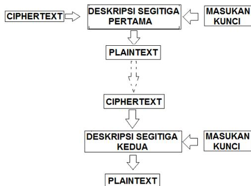
**Gambar 7.** Skema deskripsi triangle chain cipher
