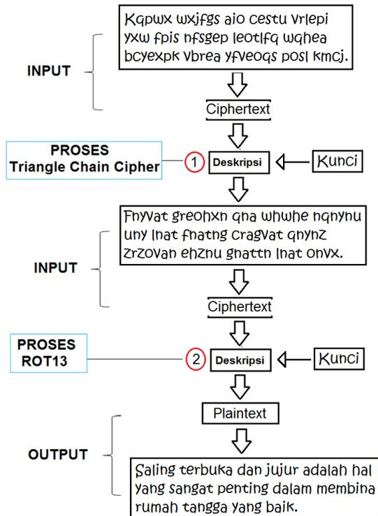
**Gambar 3.** Data input, Process and output on the process of release of password (description) text with ROT13 algorithm and algorithm of TCC
